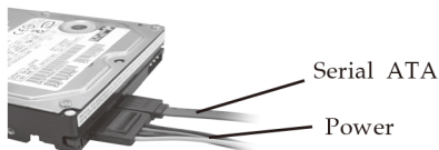
Figure 2: SATA hard disk drive connections
