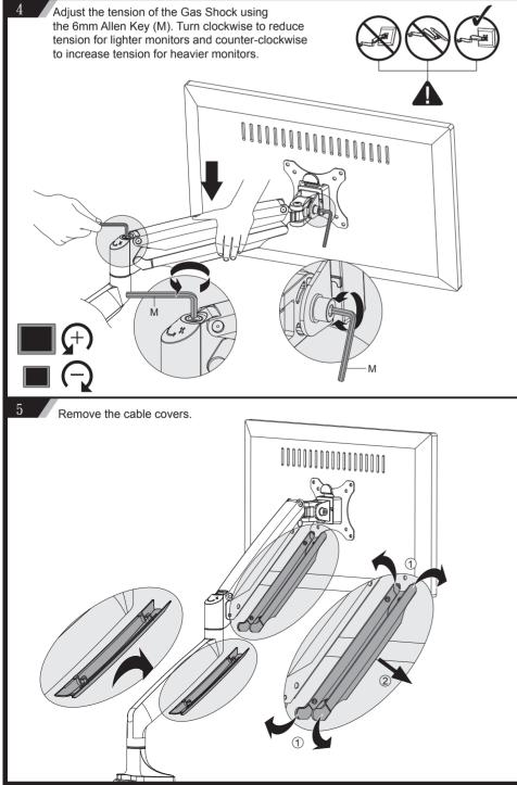
\*AVLT-Power recommends that check the mounting screws every two months for tightness.
