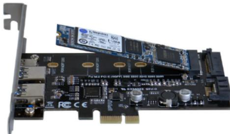
2. Secure the SSD with the included screw and nut.
